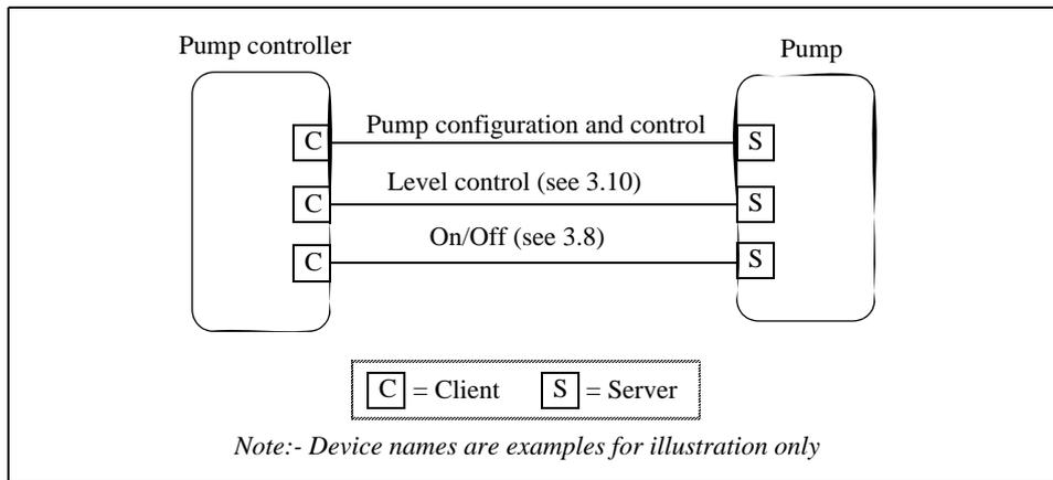
Figure 6.1 Typical Usage of Pump Config'n and Control Cluster
