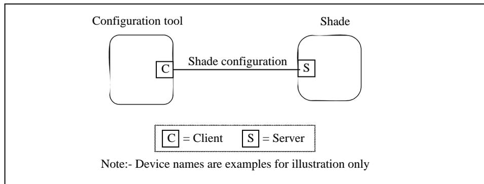
Figure 7.1 Typical Usage of the Closures Clusters
