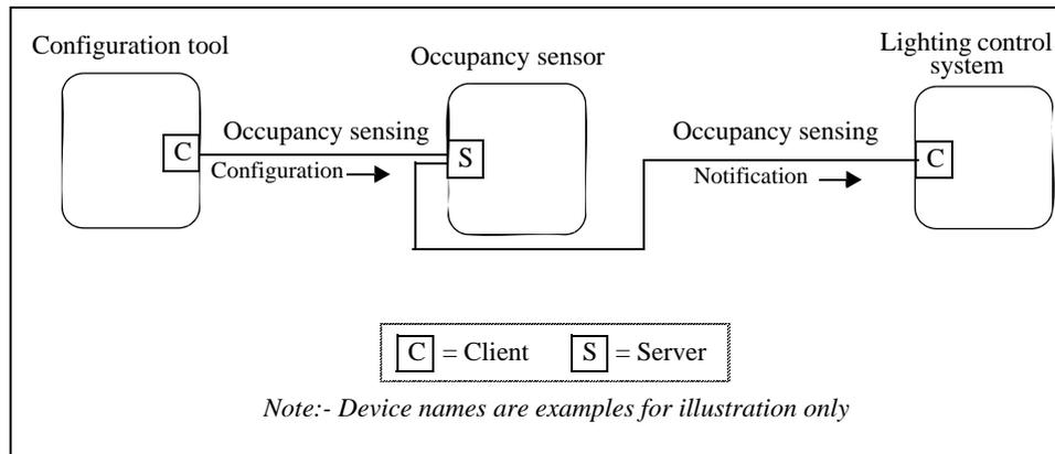
Figure 4.3 Typical Usage of Occupancy Sensing Cluster
