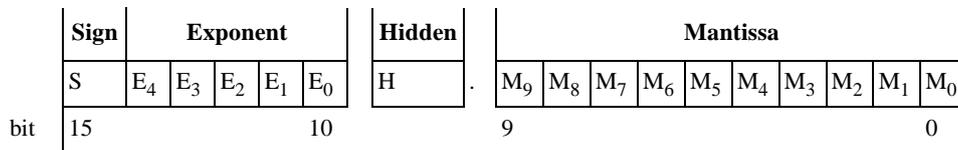
**Figure 2.36** Format of the ZigBee Semi-precision Number
